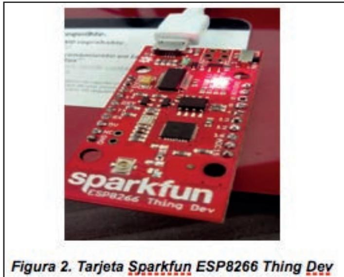
**Figura 2. Tarjeta Sparkfun ESP8266 Thing Dev**
